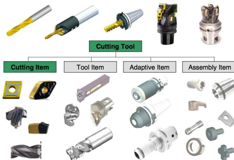
**Figure 2:** Cutting Tool Parts
